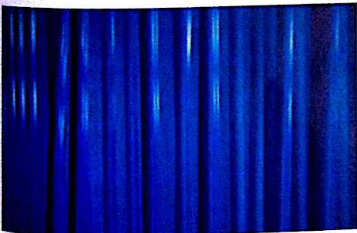
Fig. 1 10 mm thick TAKTL ® panel using the Quantz technology, integrally colored blue material.
