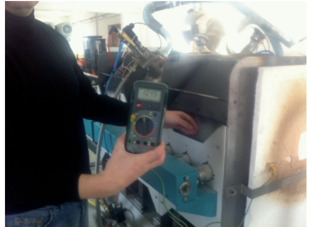
fig.: Strong isolation: Inside 1045°C, Outside 25°C
